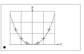
In this figure, each symmetric half of the catenary  $y = \cosh x - 1$  is approximated by a quadratic Bézier curve. The right half of the curve ends in the point (2, 2.7622), the slope there having the value m = 3.6269. Using again equation (5.1), we can calculate the intermediate control points. They turn out to be (1.2384, 0) and (-1.2384, 0). The crosses indicate points of the real catenary. The error is barely noticeable, being less than one percent.
