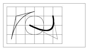
As this example illustrates, splitting up a circle into 4 quadratic Bézier curves is not satisfactory. At least 8 are needed. The figure again shows the effect of the \linethickness command on horizontal or vertical lines, and of the \thinlines and the \thicklines commands on oblique line segments. It also shows that both kinds of commands affect quadratic Bézier curves, each command overriding all previous ones.
