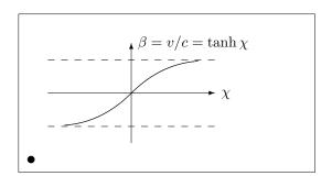
The control points of the two Bézier curves were calculated with formulas (5.1). The positive branch is determined by  $P_1 = (0, 0)$ ,  $m_1 = 1$  and  $P_2 = (2, \tanh 2)$ ,  $m_2 = 1/\cosh^2 2$ . Again, the picture is defined in mathematically convenient coordinates, and the lower left corner is assigned the mathematical coordinates (-3, -2) (black disk).
